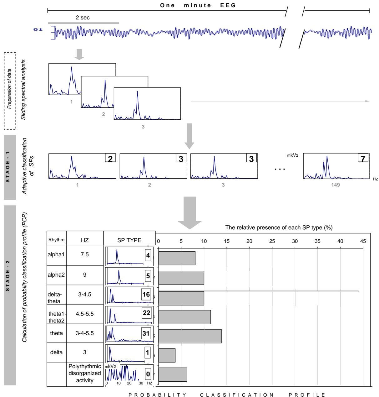
**Figure 1.** The scheme of the data processing. Sliding spectral analysis, adaptive classification of spectral patterns (SP) and calculation of the probability-classification profiles (PCP) were done separately for each subject and each channel of 1-min EEG. Reproduced from Fingelkurts et al., (2007).
