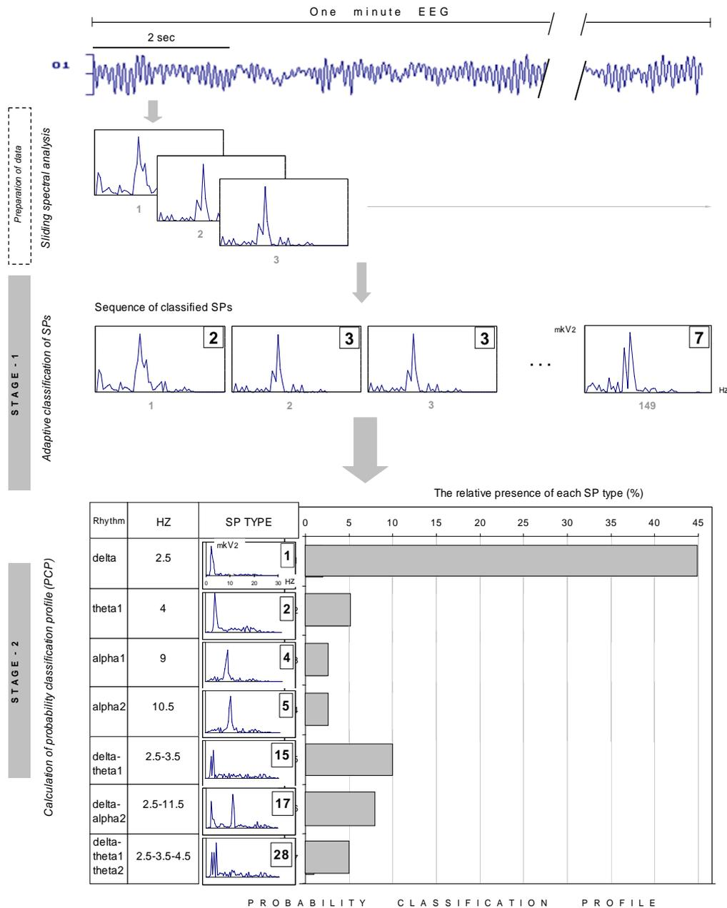
**Figure 1. The scheme of the data processing.** Sliding spectral analysis, adaptive classification of spectral patterns (SP) and calculation of the probability-classification profiles (PCP) were conducted separately for each channel of 1-min EEG (modified from Fingelkurts et al., 2006a). Gray small numbers under each SP represent the running numbers from 1 to 149. The numbers in the square represent the labels – types of classified SPs (1-32). Column “Hz” represents the
